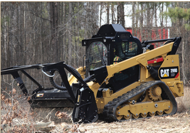
Mulchers, or masticators used for hazardous fuels reduction can clear back saplings and brush along roadways to increase line of sight and widen exit routes in preparation for an evacuation. Photo: Cassidy Bill Vaughan, DMFC Forester
